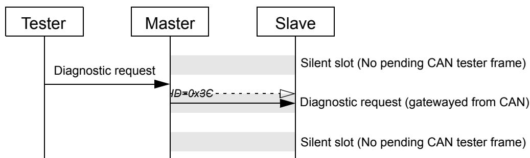
Figure 5.1: Gatewaying of CAN messages to LIN.
