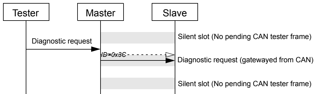
Figure 5.1: Gatewaying of CAN messages to LIN.
